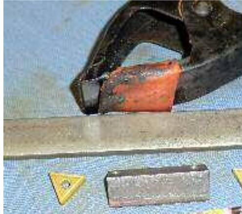
The Mark One required tapping bolt holes to secure the inserts to the angle. By clamping the angle to a flat bar, you can easily position the inserts side-by-side and flat to the bar as shown. For clarity, I'll refer to the flange of the angle with the inserts as the 'face' and the other flange as the "clamp surface". A few drops of superglue will keep them in place when you carry them over to the....
