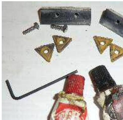
just use some spring clamps. If you do, you can blow off all the drilling and tapping to hold the inserts in place but you still need those close-fit and tapped holes in the clamp surfaces.
