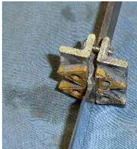
So go to the grinder, run the belt to the edge of the platen and grind away as shown. The belt won't cut the carbide (true even for ceramic belts). Make the plunge cut on one side, then flip the blade over and repeat on the other. That was EASY.
